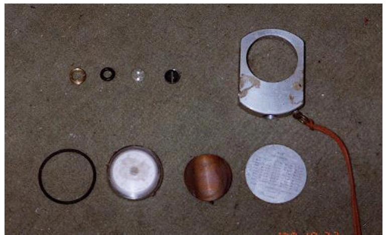
Figure 2 - The completely disassembled instrument. The top row is bush, O-ring, lens, sighting slot, body. The bottom row is O-ring, capsule, Spring-washer, Backplate
