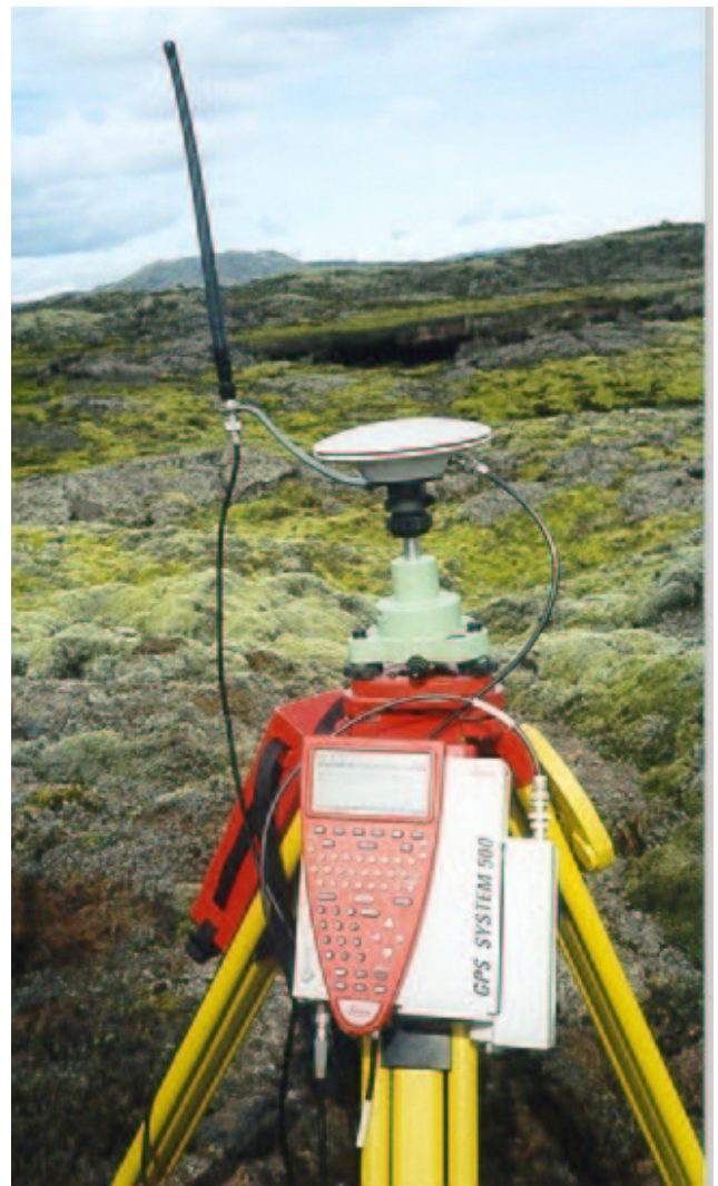
Figure 1: A DGPS Base station in use. As can be seen the base station is a large tripod mounted piece of equipment. The mobile unit is of similar size but fitted with carrying straps. [photo: Phil Collett]
