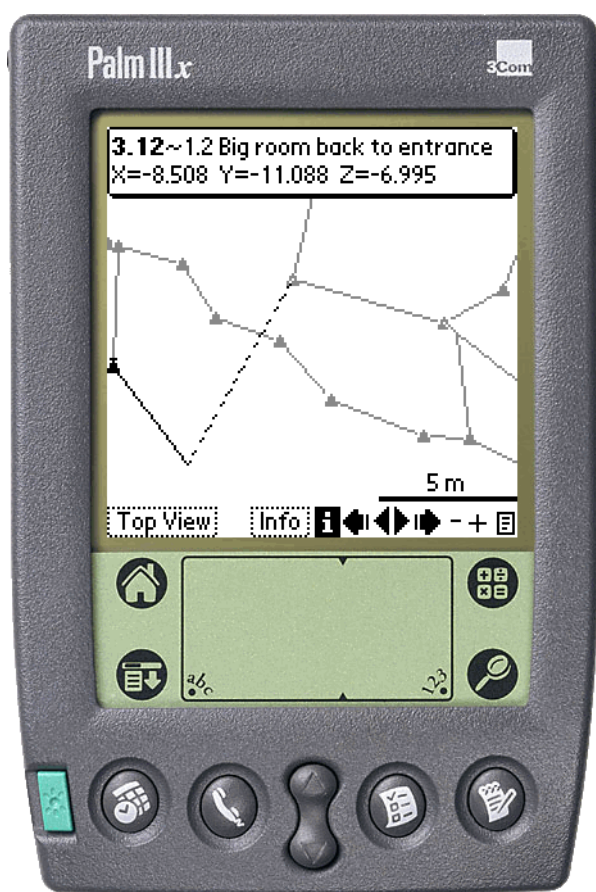
Figure 1: Palm top running Auriga: the cave map screen. Loop errors are graphically displayed with a dotted line between the actual and theoretical ends of erroneous survey shots.
